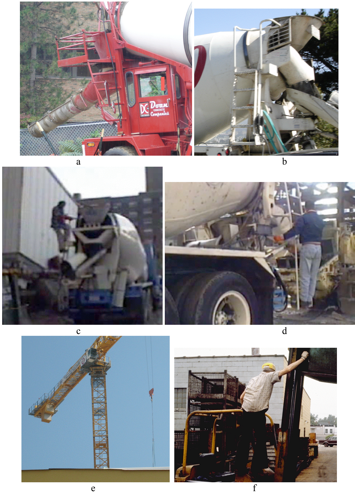
Figure 1: Examples of fixed ladders and fall hazards: ready mix truck that unloads from front (a), ready mix truck that unloads from rear (b), worker climbing up ladder on ready mix truck with hose in one hand (c), worker standing on ladder operating controls to unload ready mix truck (d), construction crane (e), worker climbing on fork lift to empty dumpster (f).
